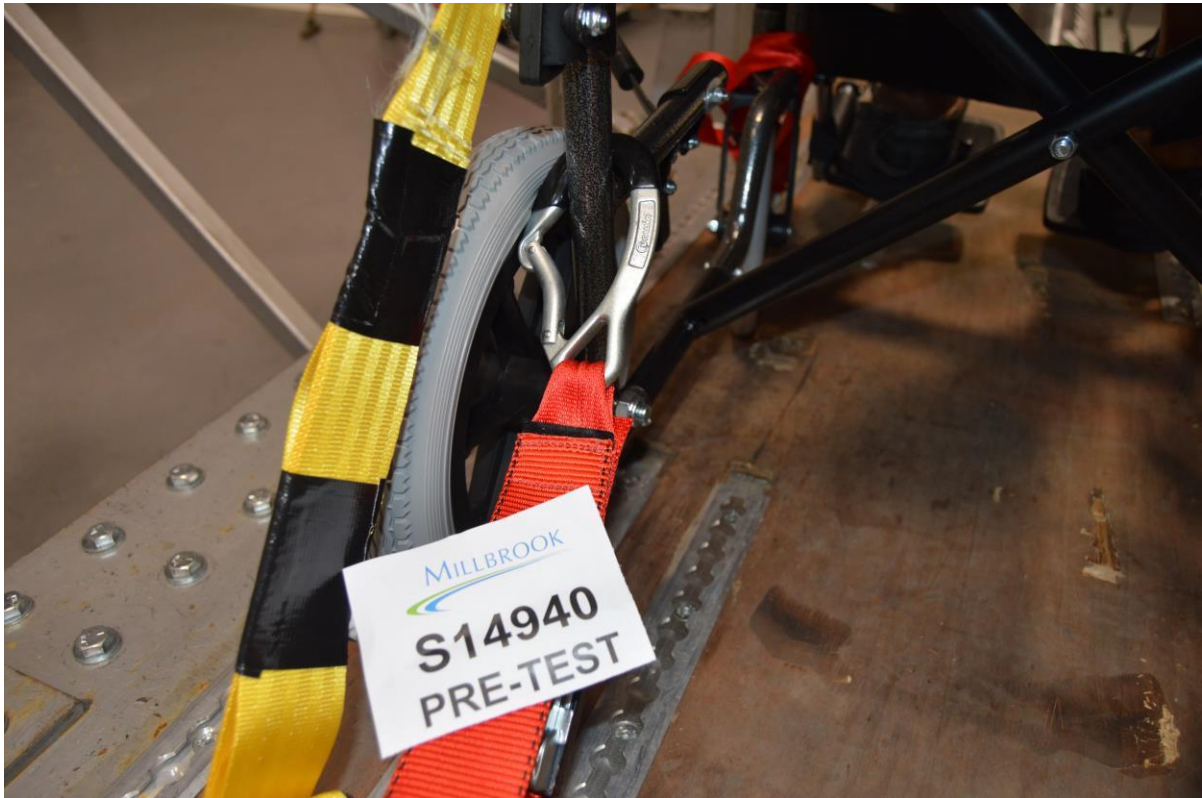
LH rear tie-downs, pre-test
