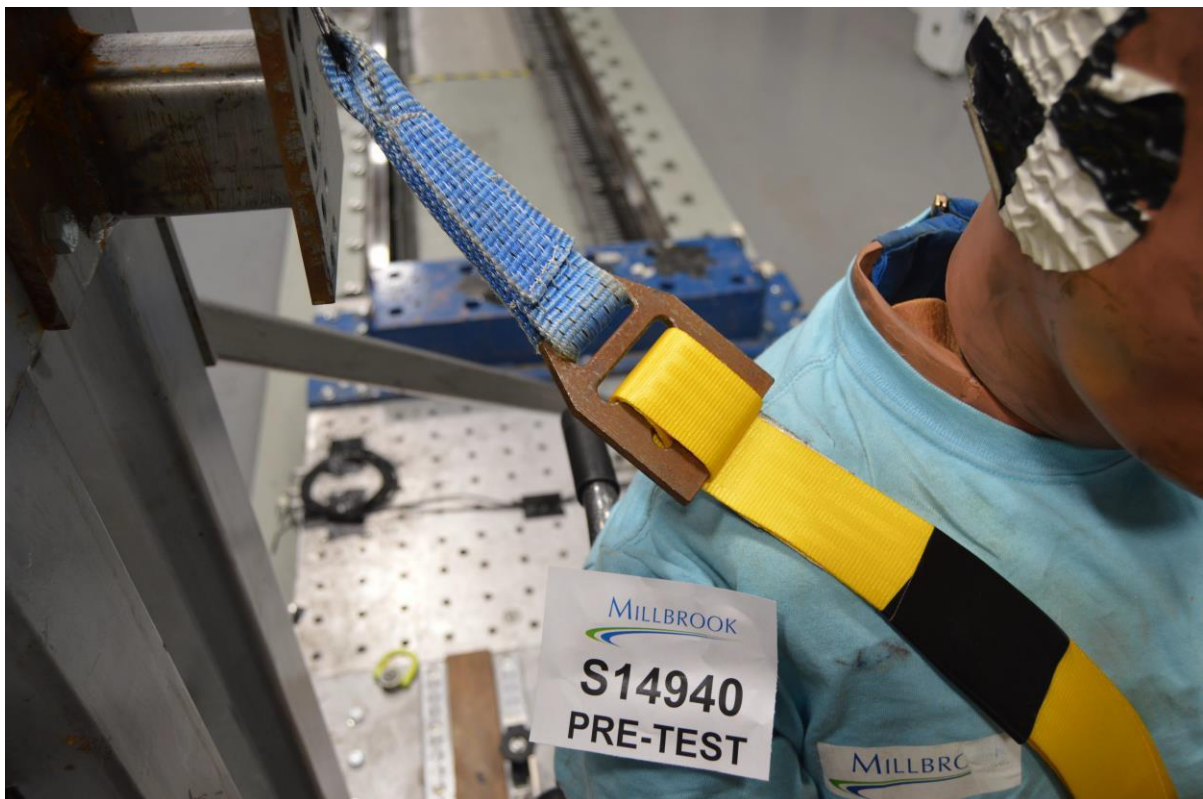
Upper torso restraint anchorage, pre-test
