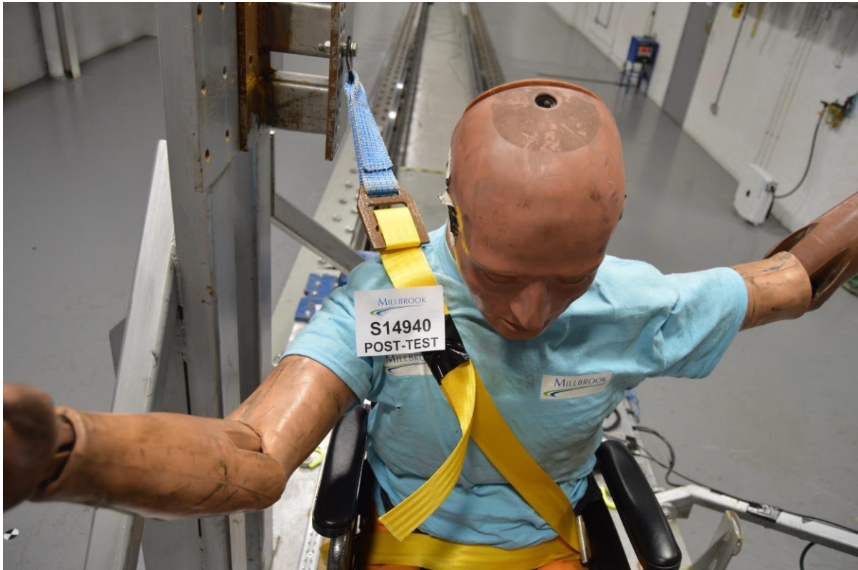
Occupant restraint upper anchorage point, post-test
