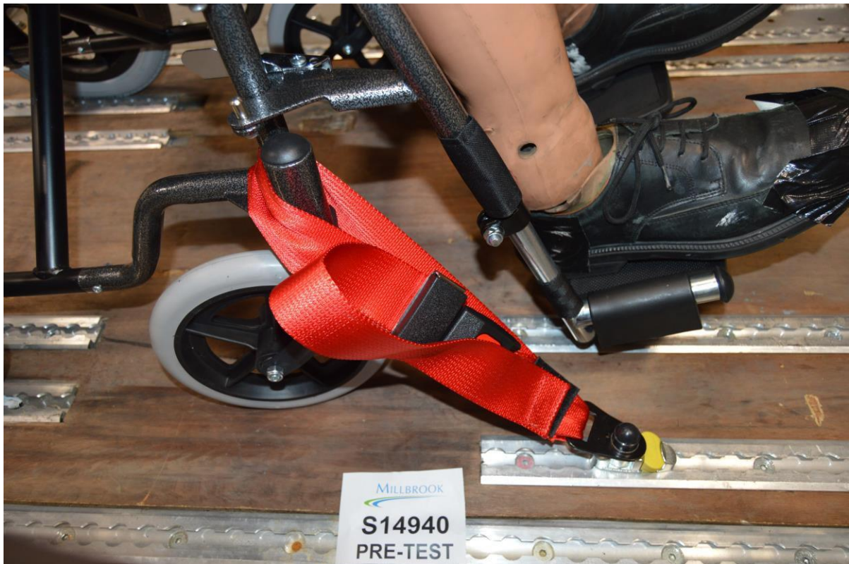
RH front tie-down, pre-test
