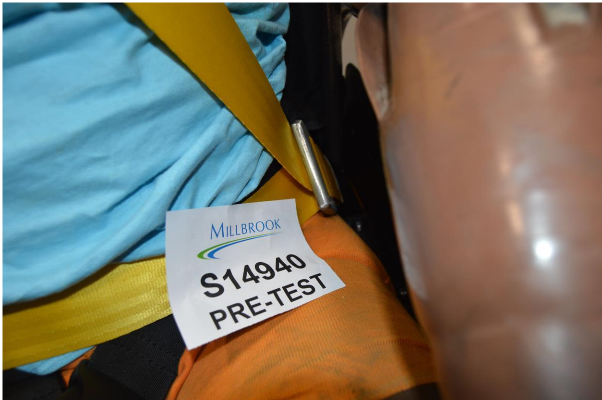
Lap belt position, pre-test
