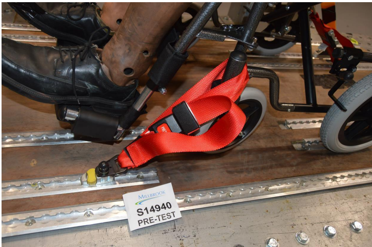
LH front tie-down, pre-test
